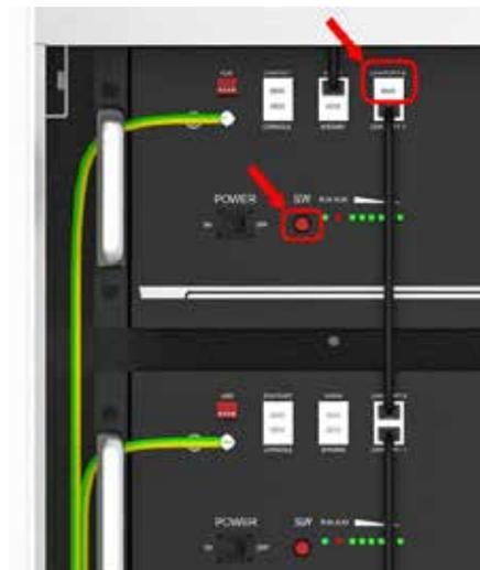
3) Press the **red SW button** of **master battery** to power on, all the battery LED light will be on one by one from the Master battery:
