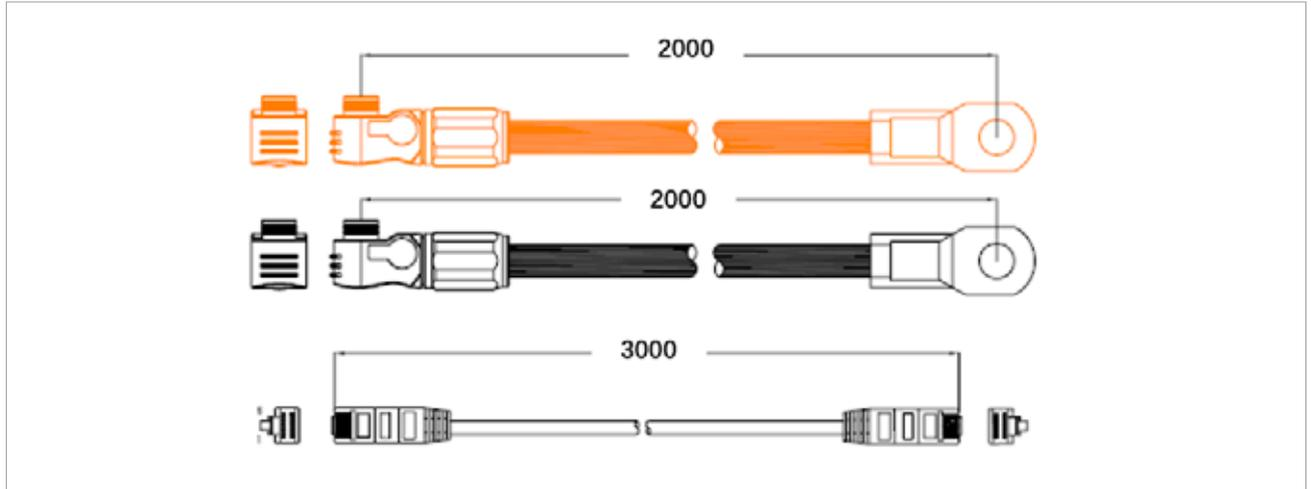
For the external cables, the length shall less than 3 meters.
