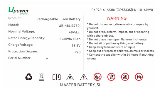
Figure1-1 Battery Energy Storage System nameplate
